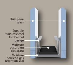
The Intercept ULTRA Stainless spacer system delivers thermal performance, structural integrity and reliability to maximize your new window investment.
